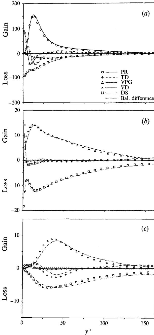
FIGURE 15. Terms in the Reynolds-stress budgets of the fluctuating velocity components in wall coordinates: (a) the streamwise velocity component, (b) the circumferential velocity component and (c) the normal-to-the-wall velocity component. The symbols denote the corresponding terms for the channel flow data reported by Mansour *et al.* (1988). The pipe flow budgets are computed from the DNS(U) data.
