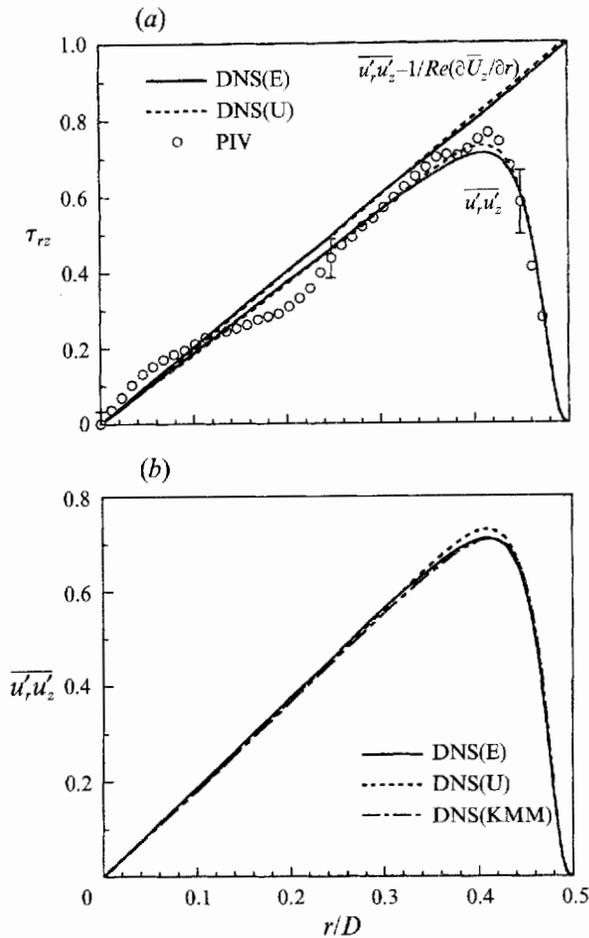
FIGURE 12. Reynolds shear stress and total shear stress distributions, normalized by the shear stress at the wall, as function of  $r/D$ : (a) the present numerical and experimental results, (b) a comparison of the Reynolds shear stress in pipe and channel (for plotting purposes, the sign of the shear stress in the channel flow has been inverted).
