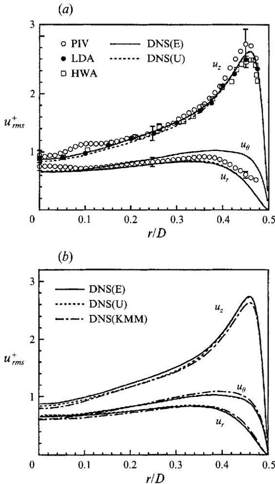
FIGURE 8. Root-mean-square (r.m.s.) velocities normalized by the wall friction velocity  $u_+$  as function of the distance from the centreline: (a) the present numerical and experimental data, (b) a comparison of the present DNS data with the DNS data obtained by KMM for their DNS of turbulent channel flow. The error bars shown for the measurements indicate the 95% reliability intervals computed from the experimental data.
