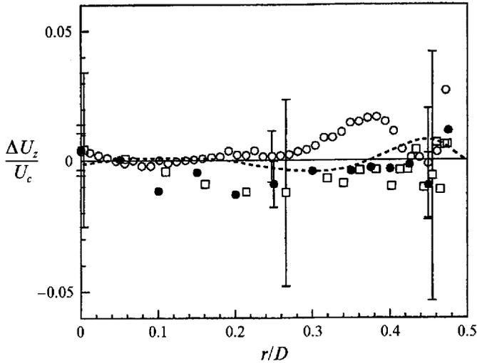
FIGURE 3. Residual mean velocity normalized by the centreline velocity  $U_c$  as function of the distance from the centreline. These residuals are computed with respect to the DNS(E) data. The error bars shown for the measurements indicate the 95% reliability intervals computed from the experimental data. For symbols see figure 2.
