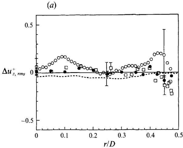
FIGURE 9. Residual axial r.m.s. velocity normalized by the wall friction velocity  $u_\tau$ , as function of the distance from the centreline. The residuals are computed with respect to the DNS(E) data. Symbols as in figure 8.
